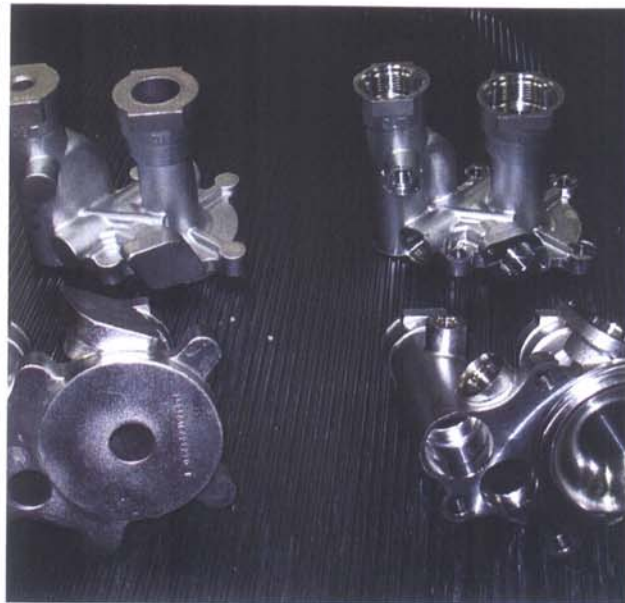
At left are the stainless steel raw castings for two complex hydraulic pump components, prior to being machined in the cell. On the right are the finished parts.
