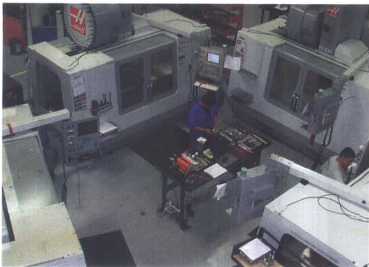
The newest manufacturing cell at Roberts Tool Co. is made up of four identical milling machines. It produces a finished complex part every 40 minutes.
